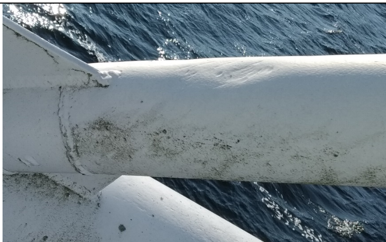
Obr. 51: Vrypy, deformace D7
